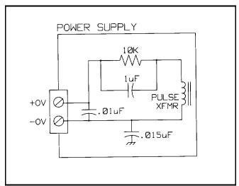
Figure 4-9. Equivalent Internal OV Trigger Circuit
